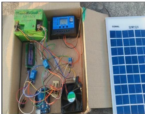
Fig 6: Recharging Battery using Solar Panel
