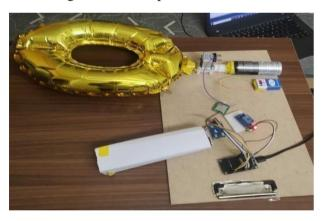
Fig 6: Making wearer afloat by sending gas from CO2 catridge to tube , When pressure Chages to abnormal conditions.
