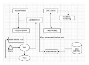
Fig 2:Conceptual Diagram of Smart Belt : IoT driven for Flotation and Real Time Monitoring
