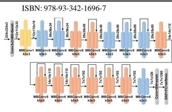
Fig. 1. Efficientnet b0 architecture
