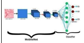
Fig 2: Architecture of MobileNet
