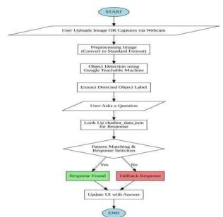
Fig. 6: Workflow Diagram of the Chatbot Operation
