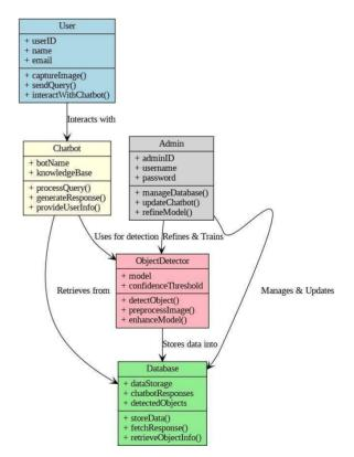
Fig. 2: UML Class Diagram of the Chatbot System
