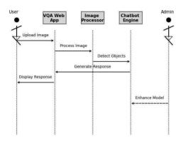
Fig. 5: Sequence Diagram of User Interaction with the Chatbot
